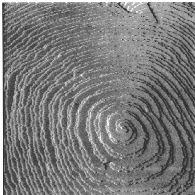
Figure 11. AFM image of a growth spiral on a canavalin crystal. Two dislocations with closely located outcrops produce two steps. A third dislocation outcrops to the upper right of these two. The steps generated by the first two dislocations propagate toward the facet periphery. Initially, the two steps are close. As they move on, the distance between them increases and becomes equal to half the spiral step. (Adapted with permission from ref 118.)
